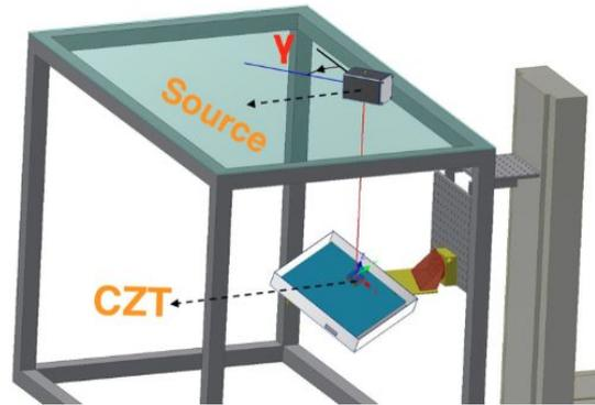
A Ba133 radioactive source to make polarized radiation.
